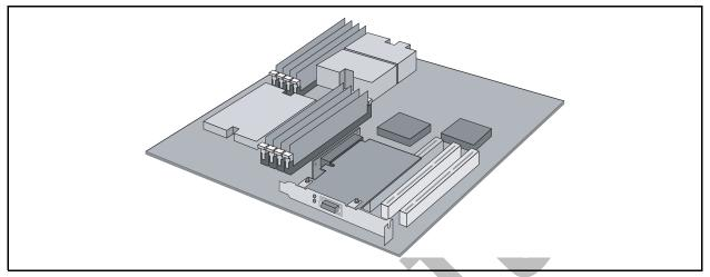
Figure 4-6. Assembled PCIe HCA with Riser
